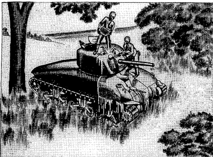
FIGURE 18.—Do not pour gasoline on tank in large quantities. It may seep into tank carrying the chemical agent along with it and also creating a dangerous fire hazard.
